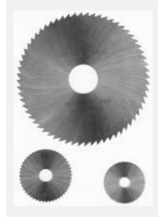
Materials: steel, cast, non-ferrous metals Application: recommended for deep slotting and cutting materials which make longer chips, suitable for cutting thickwalled profiles (wall over 2,5 mm) Machine: metal processing machines
